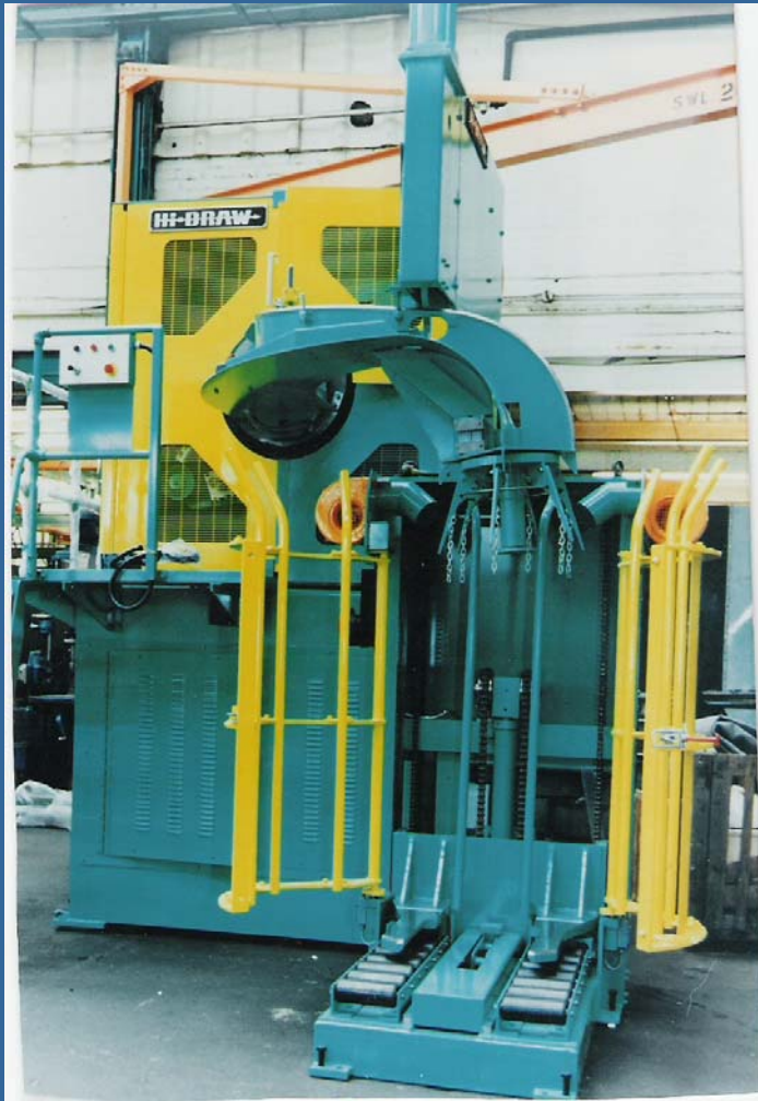
Horizontal Stator Block Coiler with pattern laying & coil lowering
